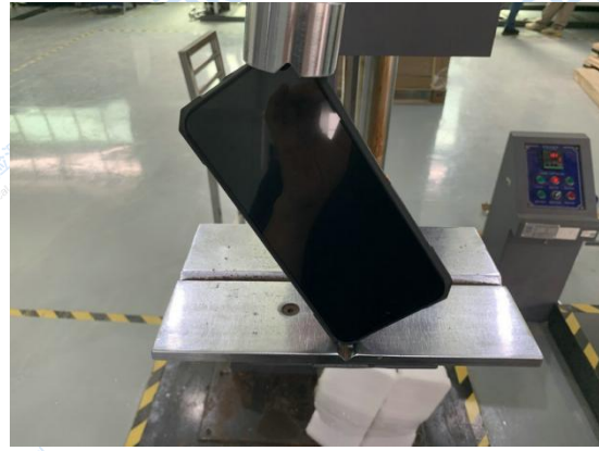
Fig.51 Test setup- Corner (4) - 5#
